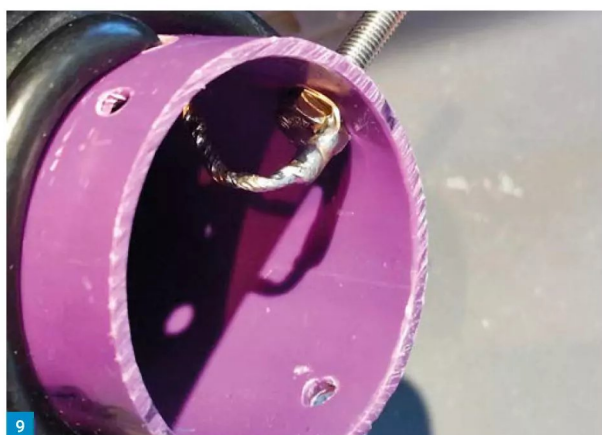
Fig. 7: The coaxial cable wound onto the former. Fig. 8: Attach shield to inner of opposite end. Fig. 9: And attach the combined connection to the ring terminal (1). Fig. 10: Attach remaining inner to ring terminal (2). Fig. 11: A diagram showing the overall arrangement. Fig. 12: Adapter for test purposes. Fig. 13: Coupling to the trap for measurement purposes. Fig. 14: Dip too high in frequency. Fig. 15: New dip after adjustment – perfect. Fig. 16: The finished trap, ready for use.
