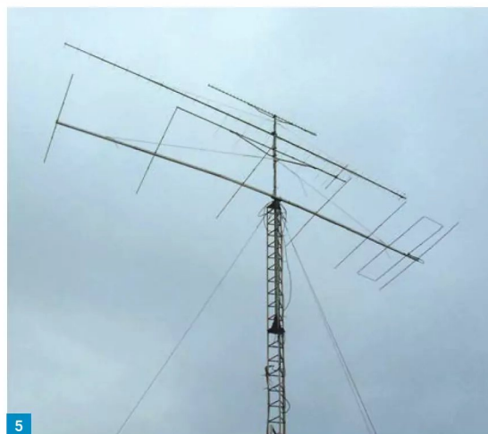
Fig. 1: The PJ4MM station is located well away from neighbours on a hilltop in the centre of Bonaire. Fig. 2: The battery room at the PJ4MM station. Fig. 3: Martin Moens PJ4MM in his VHF/UHF shack. Fig. 4: The InnovAntennas 8-element 70MHz LFA Yagi, beaming at Europe. Fig. 5: Top to bottom: 23cm 23-ele, 70cm 38-ele, 2m 9-ele and 6m 7-ele Yagis. Fig. 6: Martin building the 6m H-frame. In the background the 24m heavy-duty tower.
