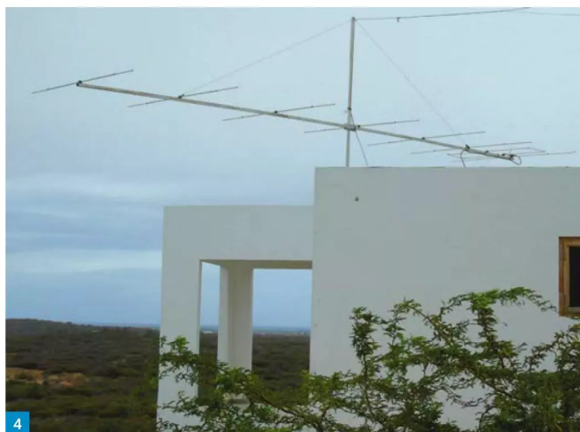
Fig. 1: The PJ4MM station is located well away from neighbours on a hilltop in the centre of Bonaire. Fig. 2: The battery room at the PJ4MM station. Fig. 3: Martin Moens PJ4MM in his VHF/UHF shack. Fig. 4: The InnovAntennas 8-element 70MHz LFA Yagi, beaming at Europe. Fig. 5: Top to bottom: 23cm 23-ele, 70cm 38-ele, 2m 9-ele and 6m 7-ele Yagis. Fig. 6: Martin building the 6m H-frame. In the background the 24m heavy-duty tower.
